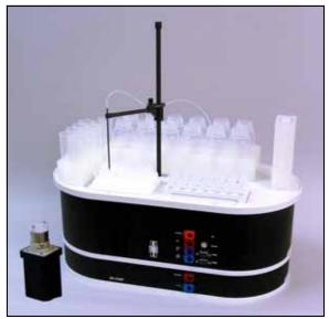
SC-FAST can be integrated to the bottom of the SC-2 for PE Elan ICPMS.
