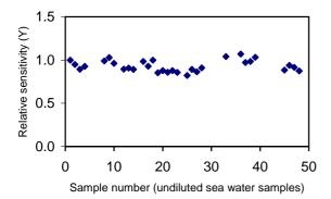
approximately 50 times with no wash or rinse steps between each analysis. Excellent precision with minimal drift can be observed.
