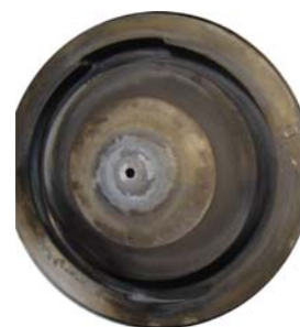
Salt free ELAN sampler cone after >300 GSL samples
